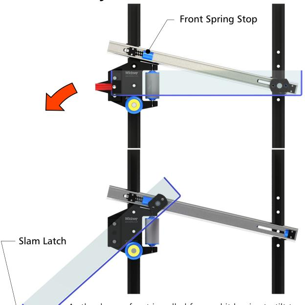
As the drawer front is pulled forward it begins to tilt towards the operator.
