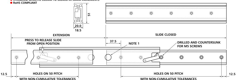
NOTE 1: 15MM DIA. HOLES IN CENTRE BEAM ALLOW EASY ACCESS TO FIXING HOLES.
