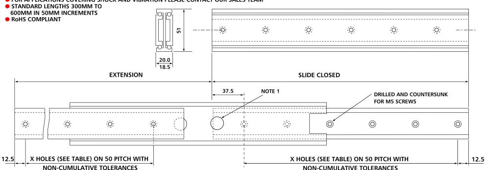
NOTE: 1. 15MM DIA HOLES IN CENTRE BEAM ALLOW EASY ACCESS TO FIXING HOLES. M5 COUNTERSUNK HEAD SCREWS TO BS4183 ARE RECOMMENDED FOR FIXING
